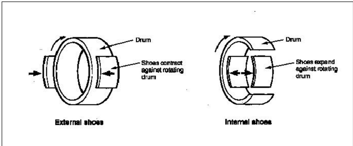
Figure 3-3. Typical shoe brakes
