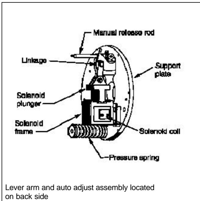
Figure 4-2. Support plate assembly
