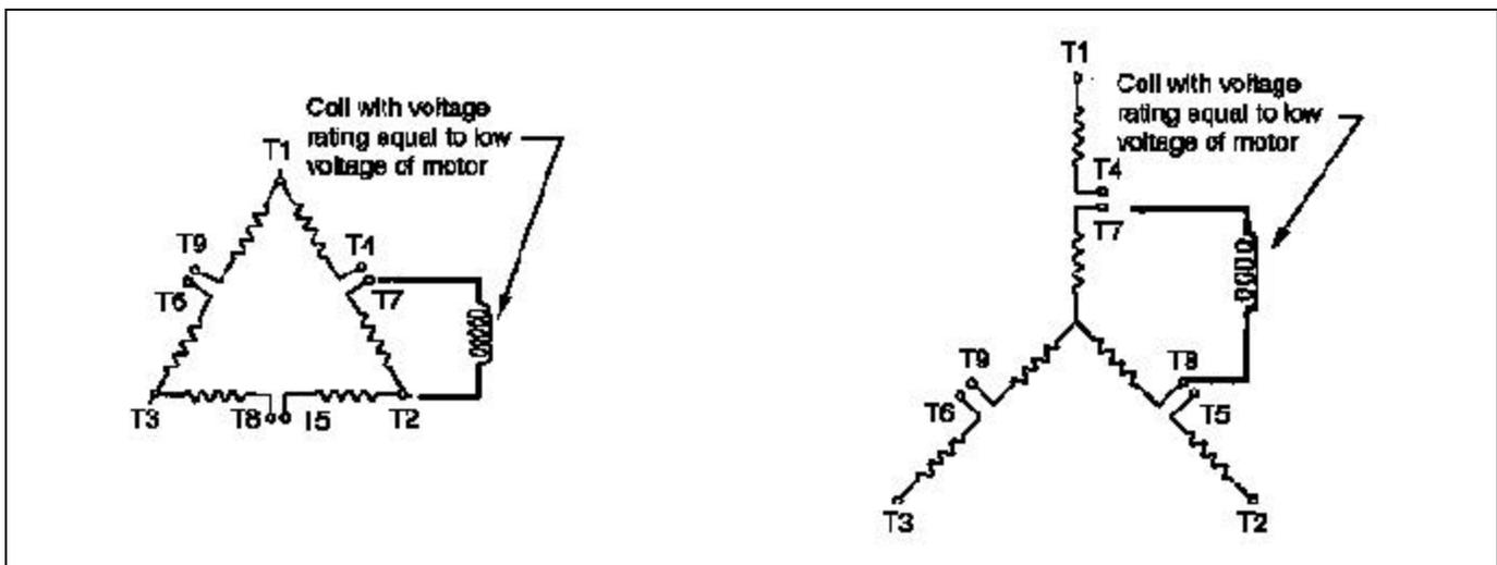
Figure 7-6. Connection to dual voltage motor
