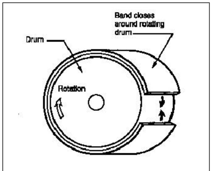
Figure 3-2. Typical band brake
