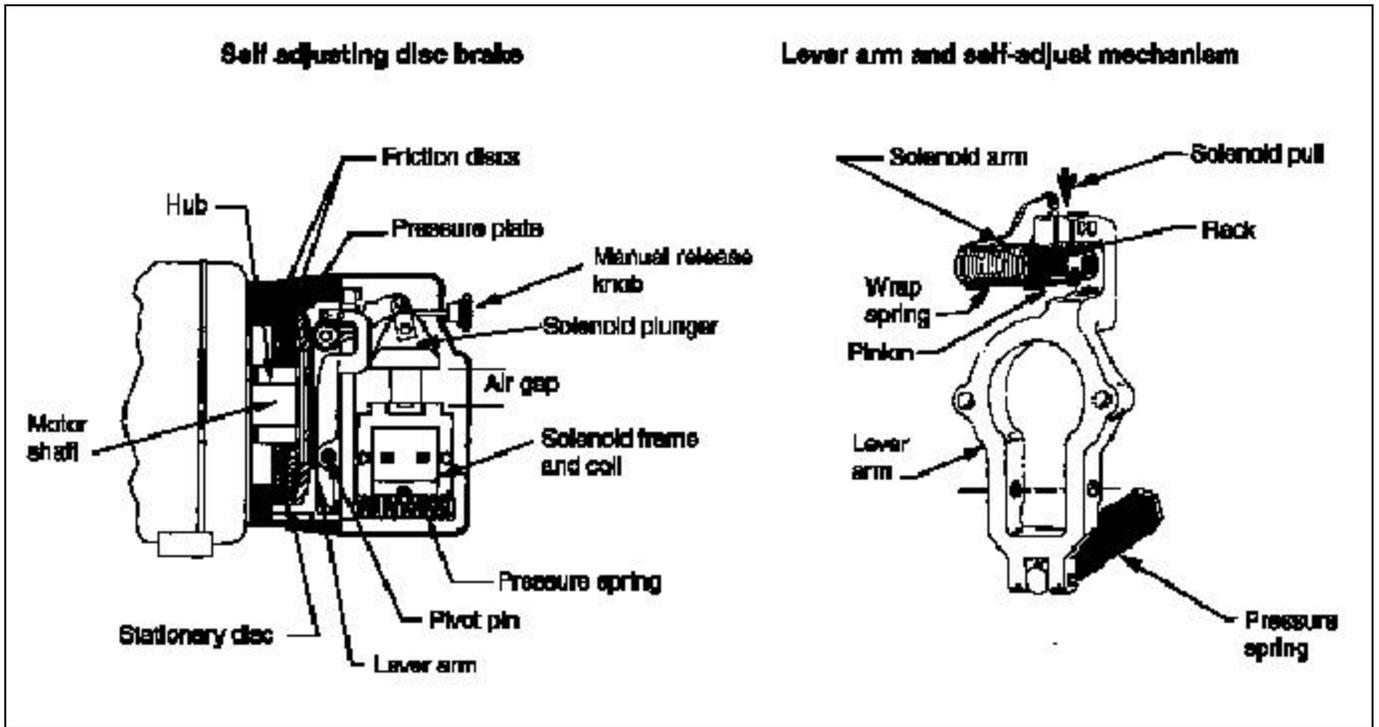
Figure 4-5. Typical Stearns self-adjusting disc brake mechanism
