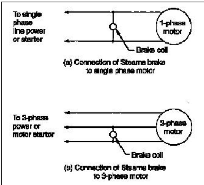
Figure 7-3. Electrical connection of Stearns brake
