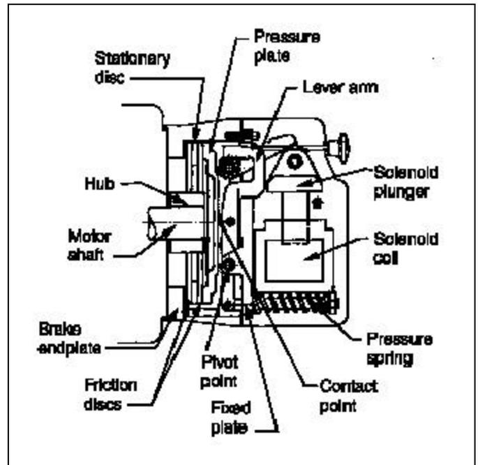
Figure 4-3. Brake in engaged mode
