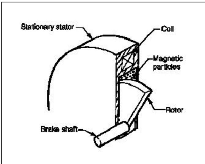
Figure 2-5. Typical magnetic particle brake
