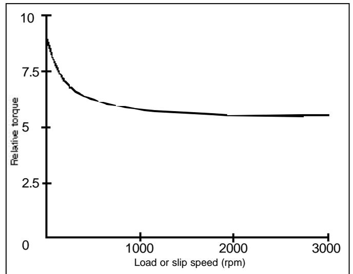
Figure 2-7. Typical torque characteristic for friction brake
