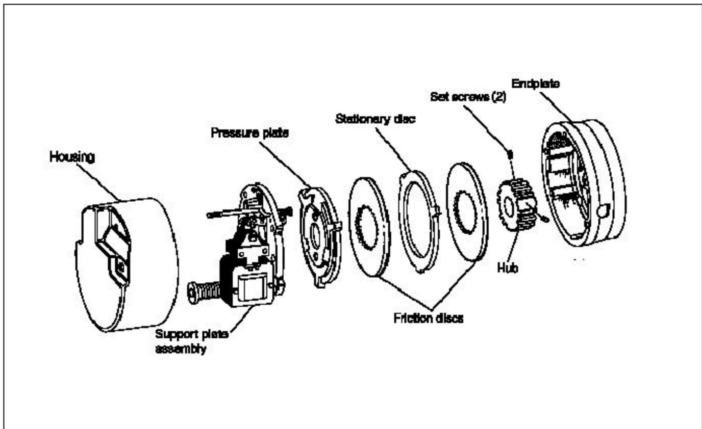
Figure 4-1. Exploded view of typical Stearns SAB brake showing basic operating components
