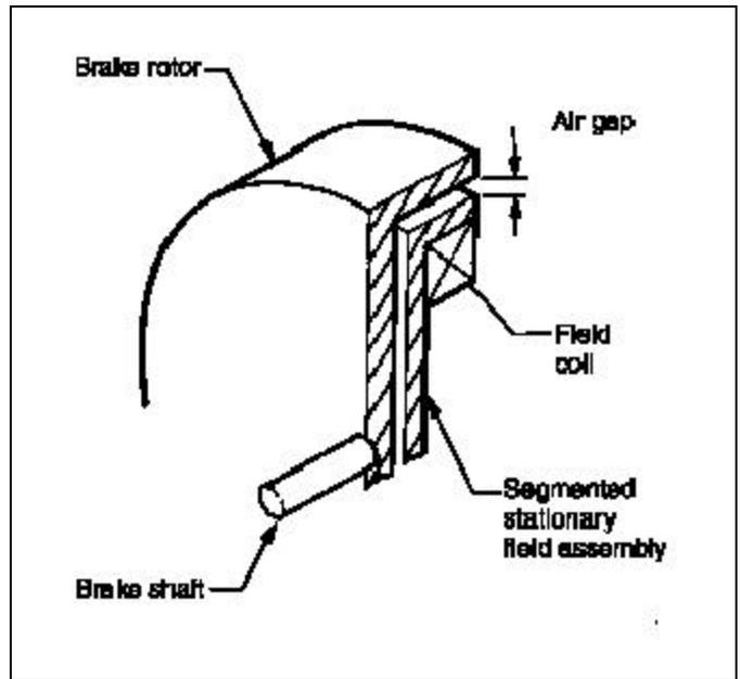
Figure 2-1. Typical eddy current brake
