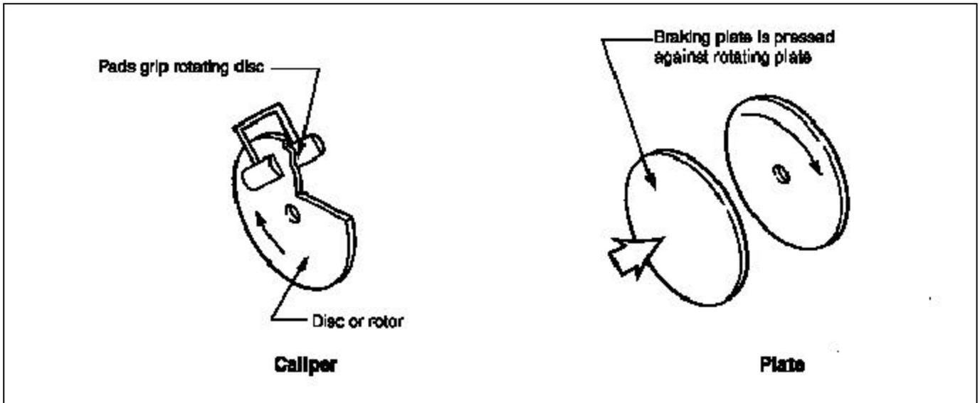
Figure 3-4. Typical disc brake types
