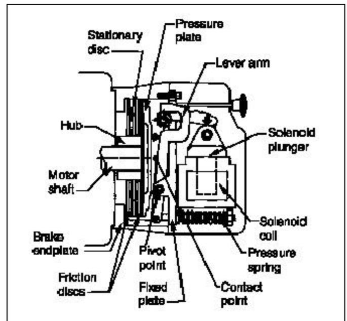
Figure 4-4. Brake in disengaged mode
