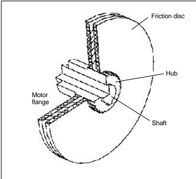
Figure 7-2. Position of hub relative to friction discs
