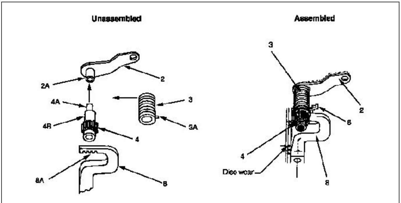
Figure 4-6. Operation of the self-adjusting mechanism
