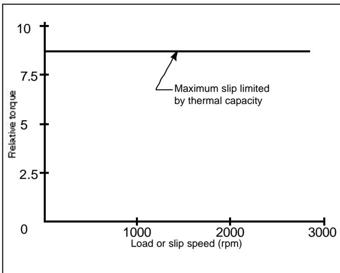
Figure 2-6. Typical magnetic particle brake torque characteristic
