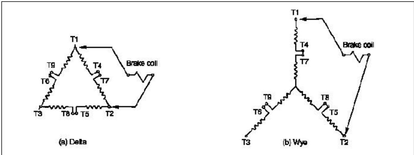
Figure 7-5. Connection to single-voltage motor
