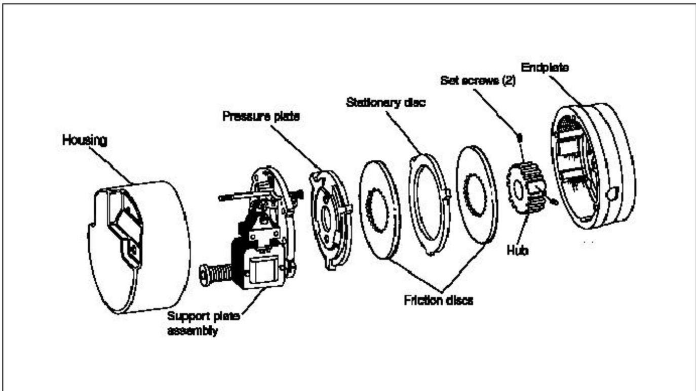
Figure 7-1. Typical arrangement of Stearns brake showing basic components
