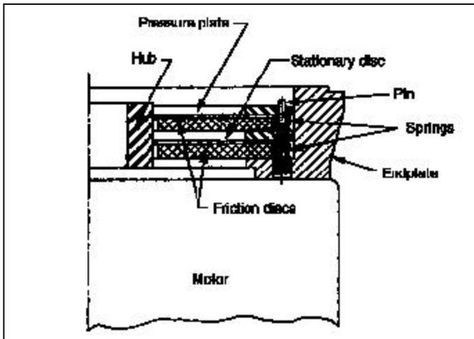
Figure 4-7. Vertical above modification, pins & springs
