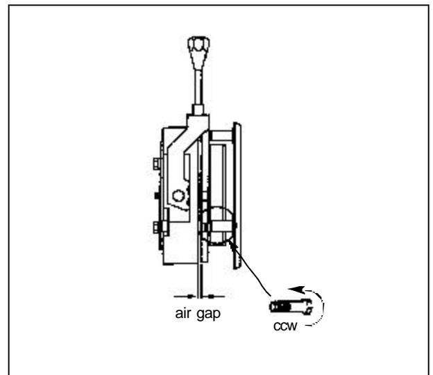
Figure 9-5. Wear adjustment– Adjustment bolts
